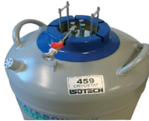
Low Temperature Measurements Facility (-180 to -80°C)
